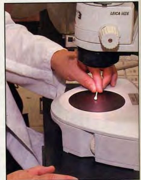
Above: Fire debris evidence collected in a metal can awaits analysis. Below: An examination under the stereomicroscope of a cotton swab for human hair.
